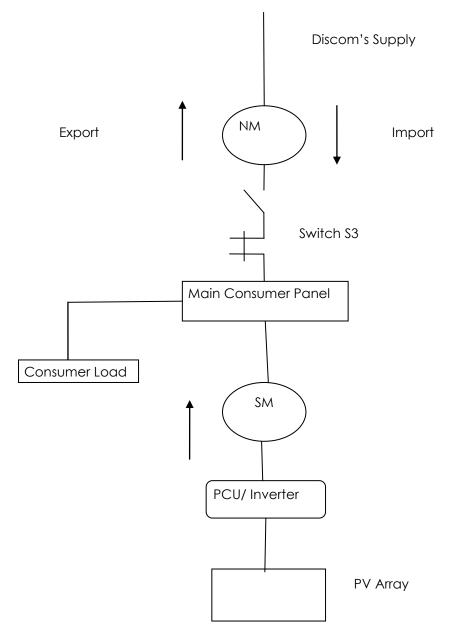
Normally, Solar Generation shall be connected with Grid. When grid fails, Inverter controlled Switch S3 Opens and on restoration of grid S3 Closes.
